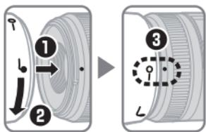
*Align the lens hood lock mark (—○) with the lens hood mounting mark (●) on the lens (③).*
